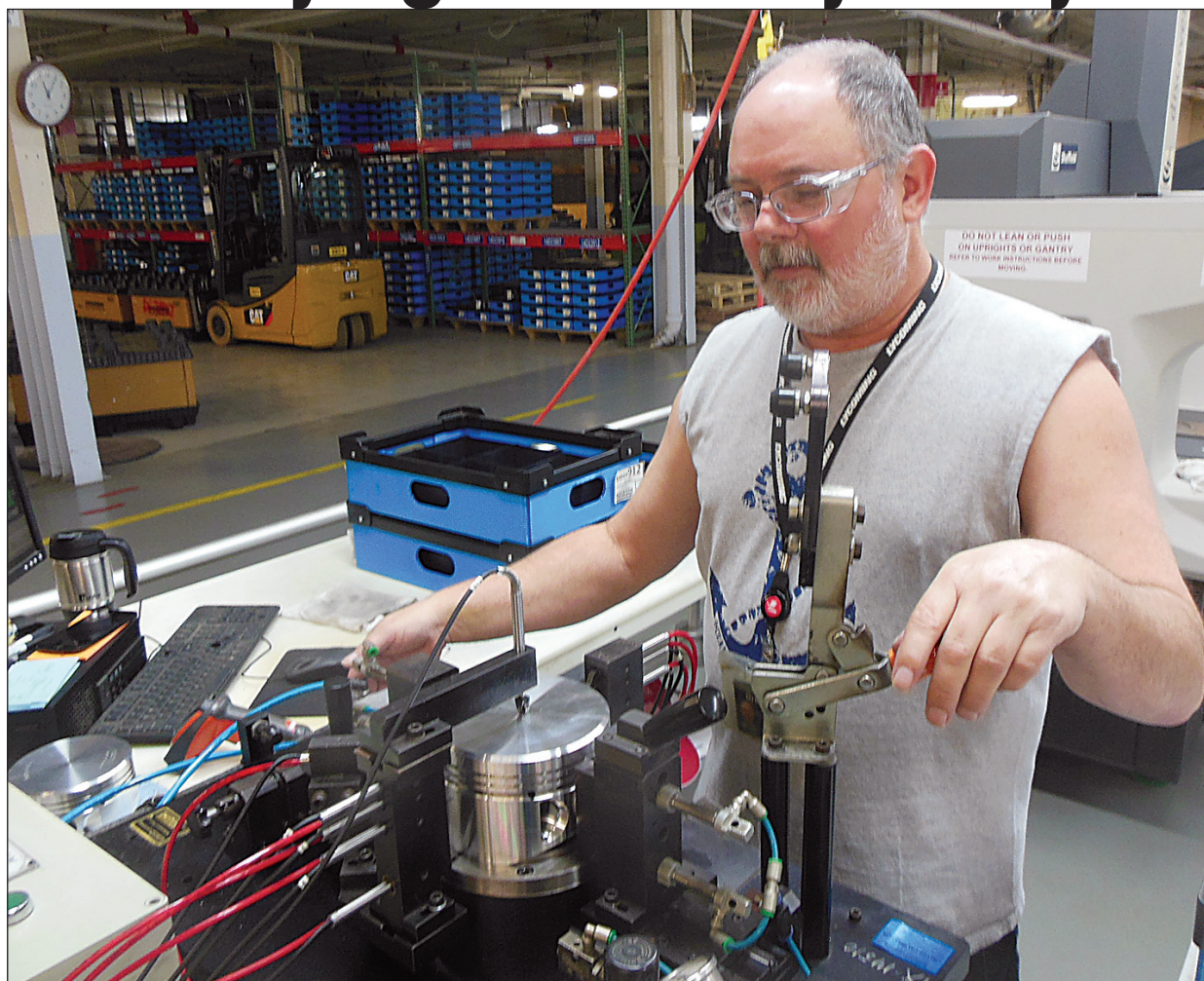
A flex cell machinist with Lycoming Engines inspects a piston.
